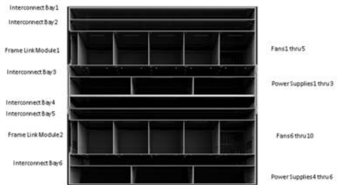
HPE Synergy 12000 Frame - Rear View
